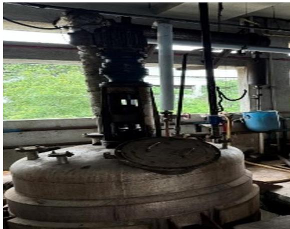
**Mixing Reactor (SS Reactor)**
