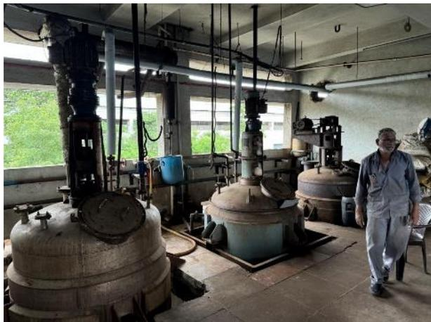
**Polymerization Reactor (SS Reactor)**
