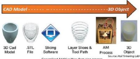
Generalized Additive Manufacturing process
