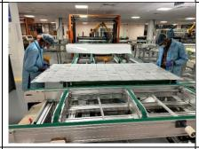
**Bussing** - After arranging strings, connect them to each other with a busbar (soldering).
