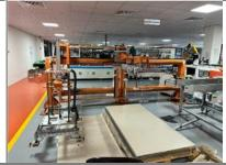
Glass Loader - Grasping mechanism will automatically draw glasses on the tray above the assembly line, automatically draw the separated paper into the recycle bin.
