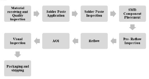
1. Material Receipt and Quality inspection – This step involve the receipt of bare PCB and other different components like micro controllers, IC, resistors, capacitors, LED, PCB and other semiconductors etc. Which are mounted on the PCB. Post the
