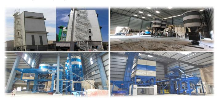
Support Equipments for Readymix Concrete Plant: Support equipments for Readymix Concrete Plant, is a facility designed to produce large quantities of concrete for construction projects, having components such as aggregate bins, powder storage silos, powder & additive weighers, batching units, mixer, control systems, screw conveyors & belt conveyors.
